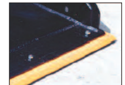
Reversible bolt-on cutting edge.
