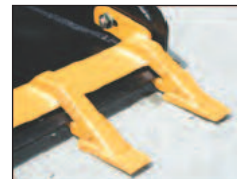
Heavy - duty bolt on Toothbar.
