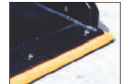
Reversible bolt-on cutting edge.
