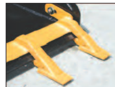
Heavy - duty bolt on Toothbar.
