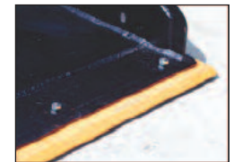
Reversible bolt-on cutting edge.
