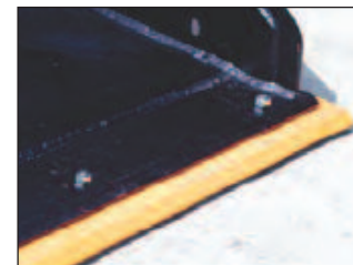
Reversible bolt-on cutting edge.
