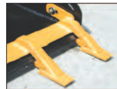
Heavy - duty bolt on Toothbar.
